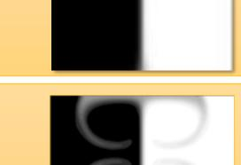
Vortex regime: double pair of steady counter-rotating vortices in the mixing channel (steady symmetric regime)
