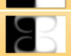
Engulfment regime: pair of steady corotating vortices in the mixing channel (steady symmetric regime)
