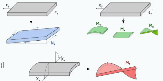
Undesired effects caused by elastic coupling terms
