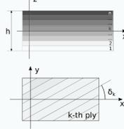
Ply indexing and layers orientations definitions in a laminate
