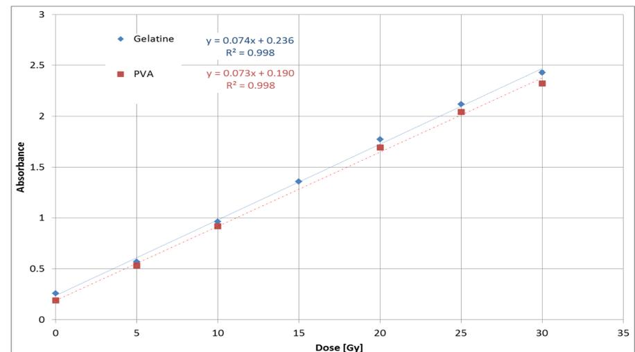
Fig.3 Comparison between sensitivity of PVA and gelatine gel
